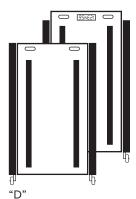
Pan dimensions 900x500 mm Weighing area 750x415 mm
