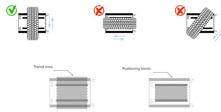
In case of wireless platforms, to preserve the correct operation of the built-in weight indicator, we recommend avoiding transit over the display, thereby preventing accidental scratches. Respect the transit area and positioning indicated in the previous drawing.
