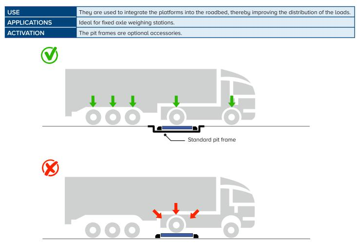
As an alternative to standard pit looms, to achieve greater flexibility in terms of use you can create a pit of an adequate length inside which you can adjust the distance between the platforms, while still keeping them at floor level:
