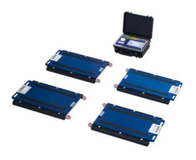
Weighs the whole vehicle and calculates the weight of the axles. Consisting of 4 WWS series portable pads and the weighing terminal with integrated printer. Wireless version.
