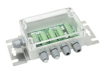
Simple junction box with IP67 protection and 4 inputs equipped with electronic board for junction of the signals of 2, 3 or 4 load cells. Screw terminal boards to facilitate the connection. The protection circuit protects against lightning and overvoltage. The reduced costs make it the ideal choice for static weighing systems such as silos, tanks and big containers.
